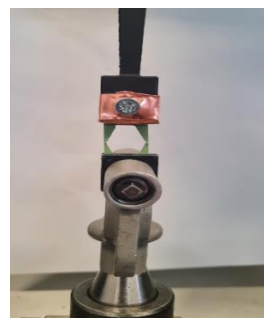
Figure 4: Tensile testing a single carbon fibre with modified top grip.
