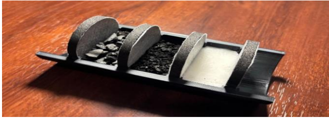
Figure 5: Photograph of the eco-friendly water filter — Visual documentation of the assembled filtration unit incorporating biochar, coconut-based activated carbon, impregnated activated carbon and bamboo charcoal filters.
